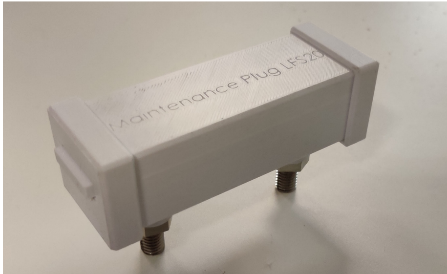
Figure 25: Prototype of the LFS20 custom Maintenance Plug
